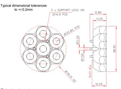
Polymer Optics "Modular LED Optics" design, based on a hexagonal format, allows maximum packing density and assembly flexibility
