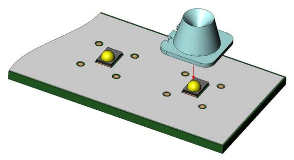
Figure 4. The square flange of the F360L-3C-S lens has 4 bumps, which should fit into 4 recesses in the PCB solder-mask.
