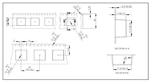
Figure 8: Tape dimensions and layout (All dimensions in millimeters)
