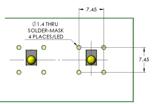
Figure 7. Dimensions and layout of the PCB location recesses used to align the lens to the LED. (All dimensions in millimeters)
