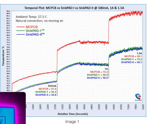
HB LEDs radiate minimal heat around the LED. Instead, all generated heat must be conducted away from the LED through the thermal pad on the bottom. By soldering the LED thermal pad directly to the aluminum base, a **Direct Thermal Path** is established that efficiently conducts the heat to the cooling surface.
