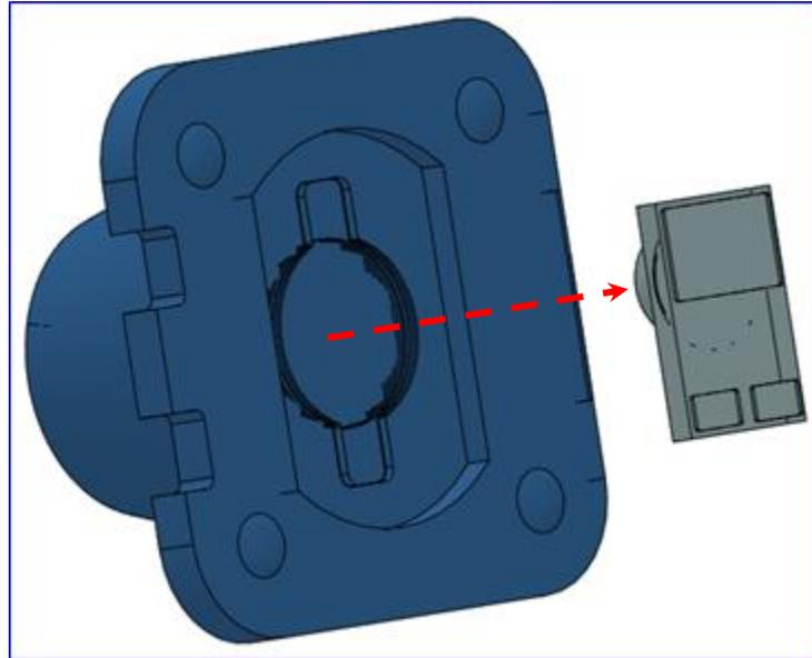
**Figure 3.** The center of the F360L-3C-SS lens should be aligned with the center of the LED dome lens. There is sufficient package clearance in the bottom of the F360L-3C-S lens to accept the rectangular LED package.
