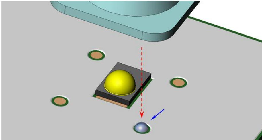
**Figure 5.** A small droplet of glue is placed at each of the 4 solder-mask recess locations, to bond the 4 lens “bumps” to the PCB. A fixture or automated placement machine will be required to assure proper lens location (to center the lens to the LED die).
