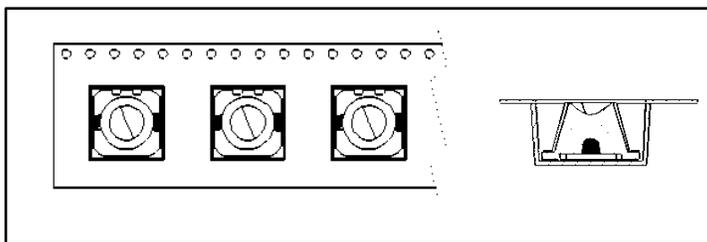
Figure 9: Orientation of lens in tape pockets
